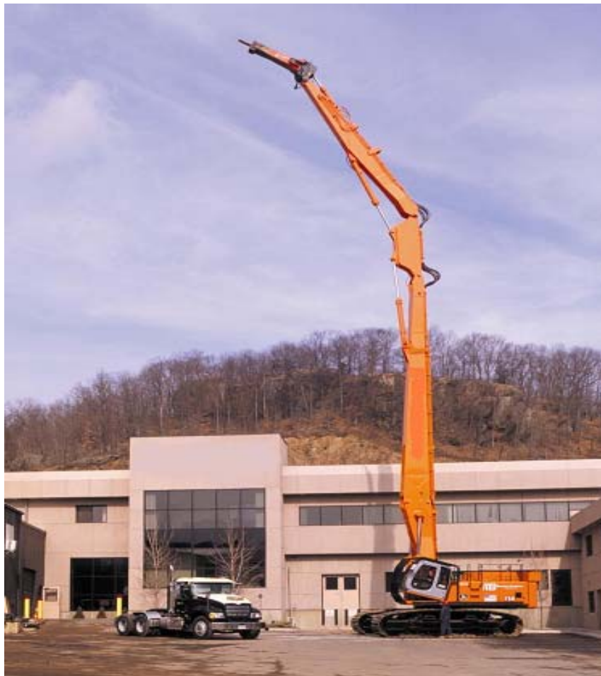
Figure A.7. Excavator and Long Reach Boom with Demo Hammer Attachment
