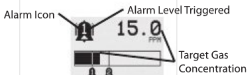
Figure 34. General Status Alarm - detail
