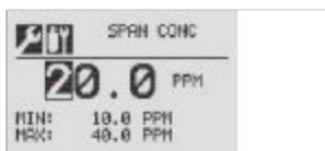
Figure 45. Span Gas Concentration screen
