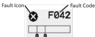
Figure 33. General Status Fault - detail
