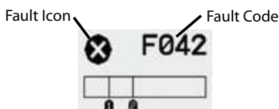
Figure 33. General Status Fault - detail
